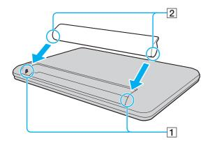
4 Push the battery pack down into the compartment until it clicks into place.
